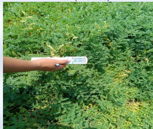
Chickpea canopy temperature observation using Infrared thermometer
