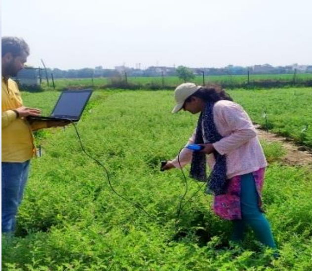
Spectral reflectance measurement of chickpea
