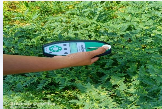
Chickpea CCI Observation using SPAD Meter (MC-100)
