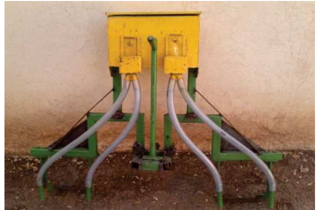
Single Bullock Operated Twin Ferti Hoe
