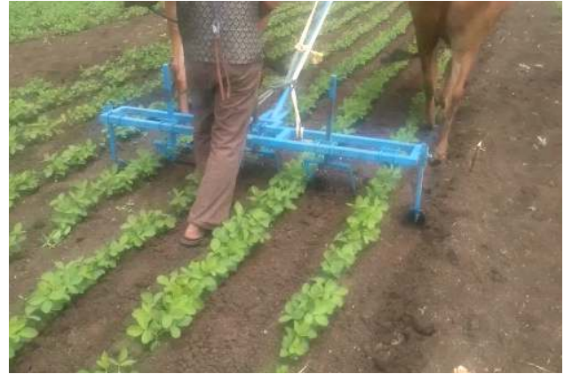
Three Tyne Hoe with Furrow Opener
