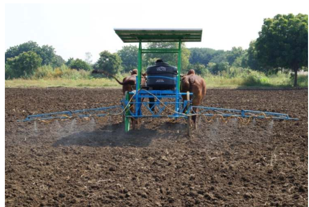
Bullock Drawn Solar Operated Sprayer
