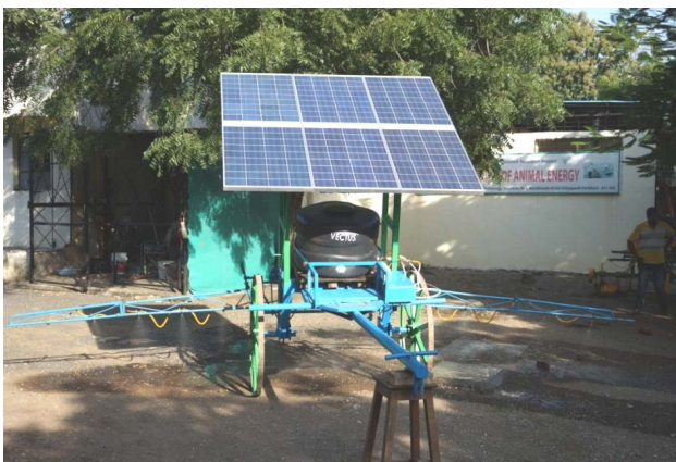
Bullock Drawn Solar Operated Sprayer
