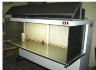
Laminar air-flow cabinet
