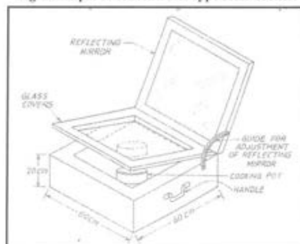
Fig. Details of a box type cooker.
