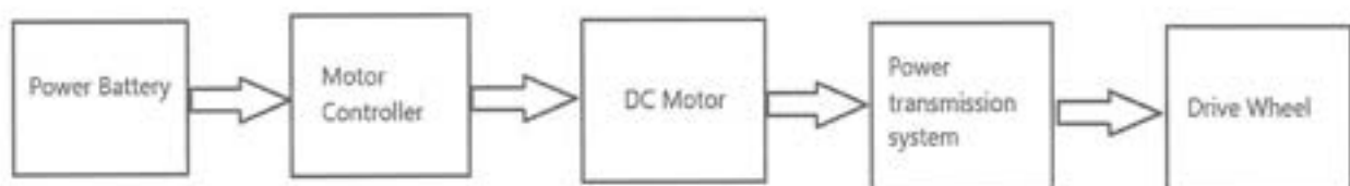
Fig. 1 : Schematic sketch of driving system for BEV weeder.
