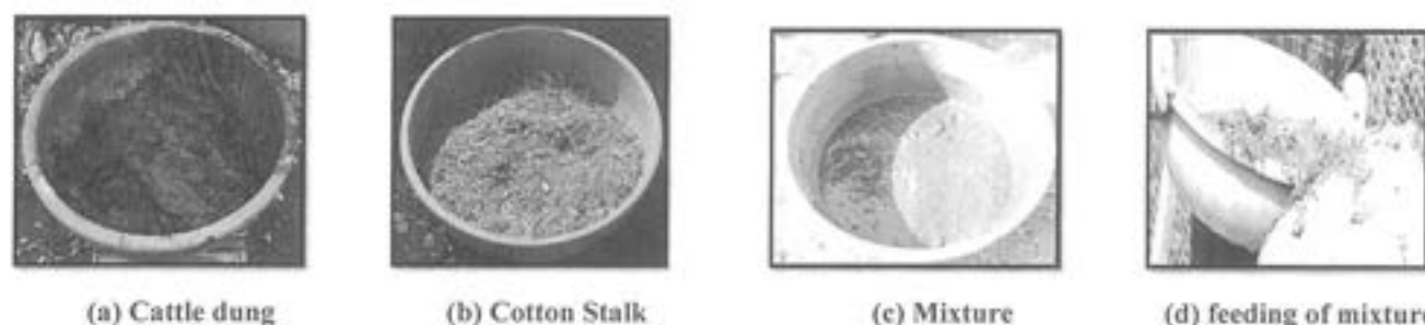
Fig. 6 (a) (b) (c) (d) Feeding of cattle dung inoculated with shredded cotton stalks
