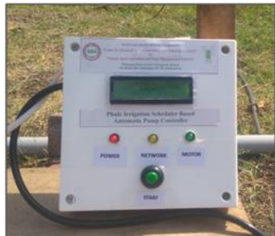
IoT based Automatic Pump Controller
