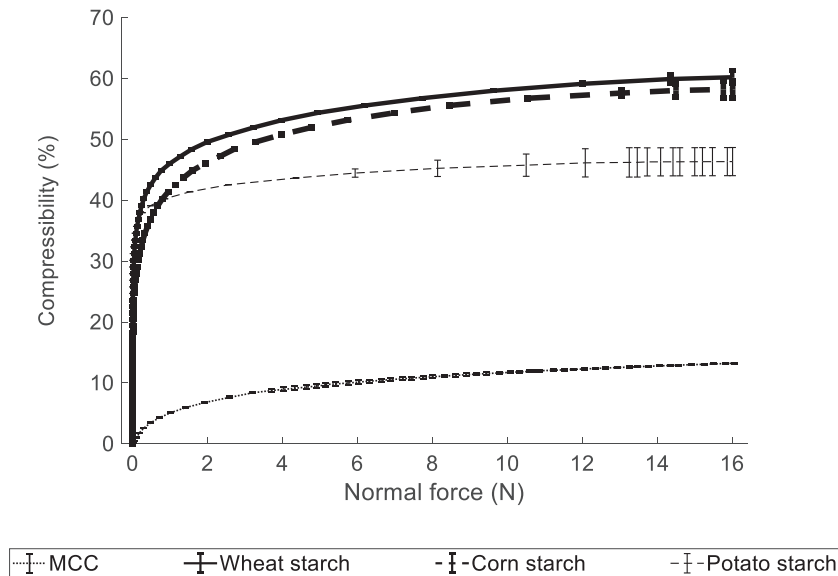
Fig. 4. Compressibility profile of powder samples.
