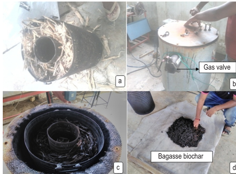
Fig. 1: Sugarcane bagasse biochar production using the electrical heating kiln (a) biomass holding chamber; (b) coverlid of kiln; (c) removal of biochar and (d) bagasse biochar.
