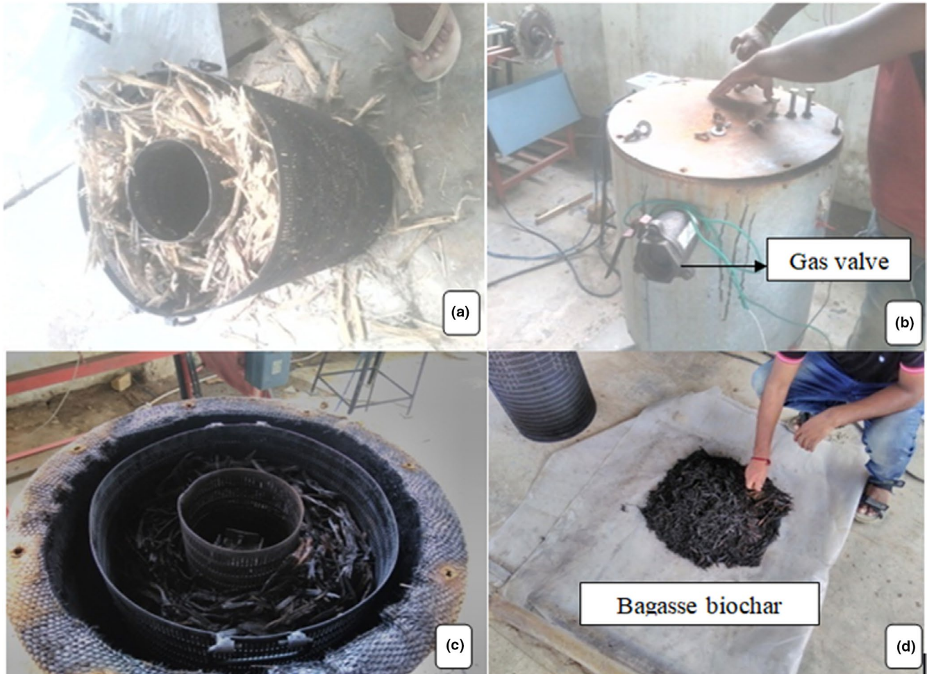
FIGURE 1 Biochar preparations in the electrical heating kiln (a) biomass holding chamber. (b) coverlid of kiln. (c) removal of biochar. (d) bagasse biochar
